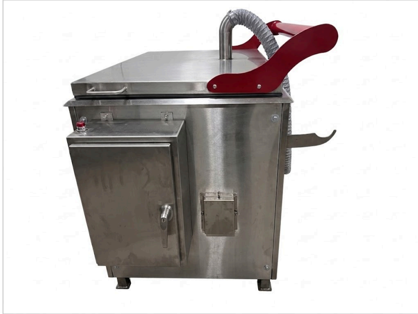
Figure 3. Secondary junction enclosure panel ("snap disc panel"), next to the main control enclosure. The bolted stainless steel panel is secured by 4 nuts and provides service access to the smaller NEMA 4X enclosure that houses the snap disc and heater wire terminations. The red light on top of the main enclosure (upper left) is the controller alarm light. The panel is on the same side as the bracket/handle hook used for forklift handling. Earlier build shown with the steel counterbalance lid arm.
