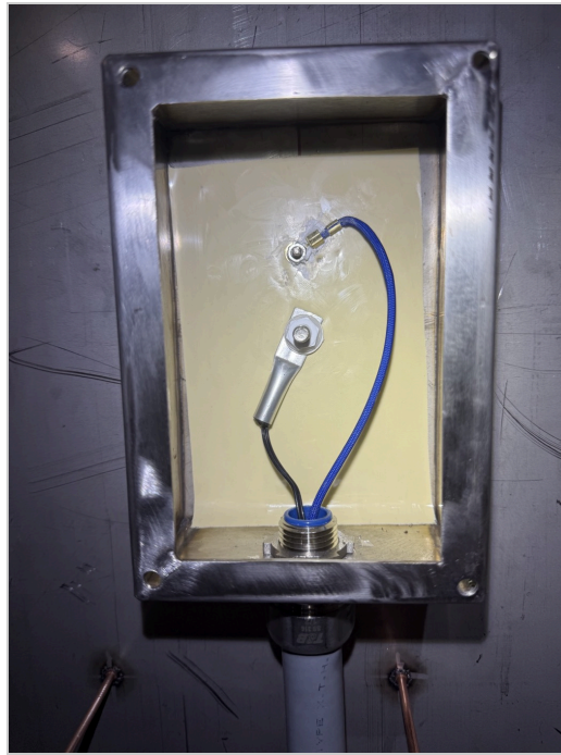
Figure 5. Redundant thermistor probe enclosure on the tank exterior. Two lug-style probes are bolted to the stainless tank wall through silicone thermal pads (cream-colored backing). The blue-jacketed loop is the nickel-plated copper lead from one probe; the second probe attaches at the lower-left lug and is aluminum, galvanically separated from the stainless steel tank. Probe leads exit through a liquid-tight conduit fitting at the bottom of the enclosure and return to the controller via the vapor-tight FMC. Disconnect both leads before measuring resistance using the table in Section 4.4.
