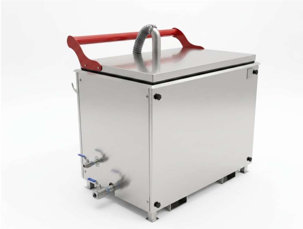
Figure 7. Drain side of the WL4 tank, opposite the control enclosure. Upper valve: 1" maintenance drain (used for routine liquid removal during sludge service or relocation). Lower valve: 2" sludge drain (used to discharge accumulated coating residue from the tank bottom). Both valves are 316 stainless steel ball valves. The 3" PTFE-lined chimney vent is visible on top.
