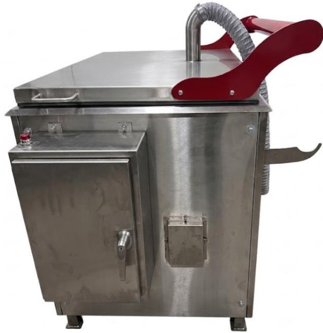
Figure 4. Secondary junction enclosure panel ("snap disc panel") mounted to the tank interior and accessible through the exterior panel, next to the main control enclosure. The bolted stainless steel panel is secured by 4 nuts and provides service access to the smaller NEMA 4x enclosure that houses the snap disc and heater wire terminations. A small red indicator on the upper face shows the snap disc status. The unit is mounted on the same side as the bracket/handle hook used for forklift handling.
